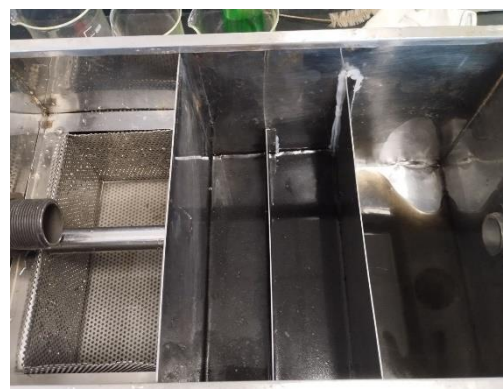
Plates 3. 2 Restaurant Wastewater in Modified Grease Trap
