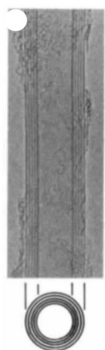
Fig. 3. One of the electron micrograph images of the microtubule structure obtained in the first report of CNT discovery comprising of five graphitic walls with a diameter of 6.7 nm
