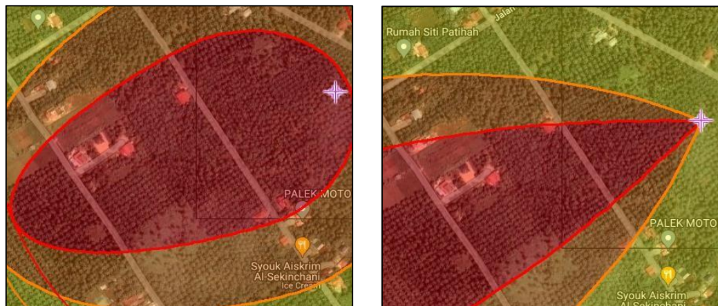
Fig. 8. (left) Footprint of H 2 released as VCE at daytime for plant 1, 160 mm leakage with 33.67% fatalities (from ENE wind direction); (right) Footprint of H 2 released as VCE at night-time for plant 1, 160 mm leakage with 11.62% fatalities (from ENE wind direction)
