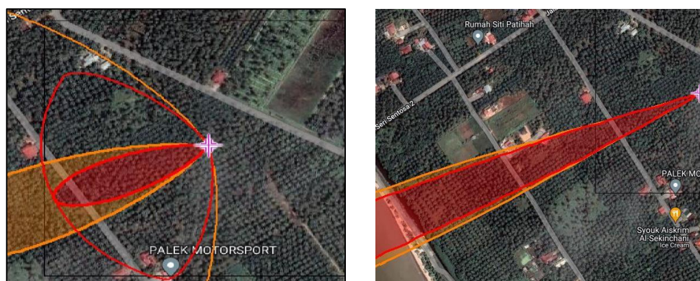
Fig. 4. (left) Footprint of CO released at daytime for plant 1, 10 mm leakage with 5.06% fatalities (from ENE wind direction); (right) Footprint of CO released at night-time for plant 1, 10 mm leakage with 3.23% fatalities (from ENE wind direction)
