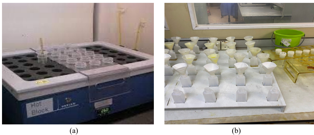
Fig. 3. (a) Heat block heating process and (b) filtration process
