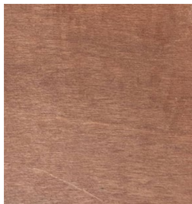
Fig. 1. Sample of plywood surface coated with control shellac
