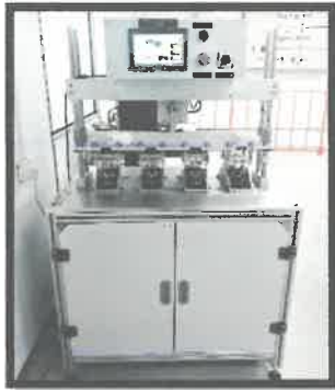
Figure 16: Main-Key Life Test
