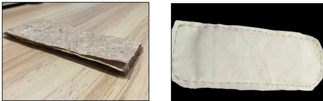
Figure 2.: Left: banana fibre sheets, right: example of a finished product of sanitary pad from banana fibres.
