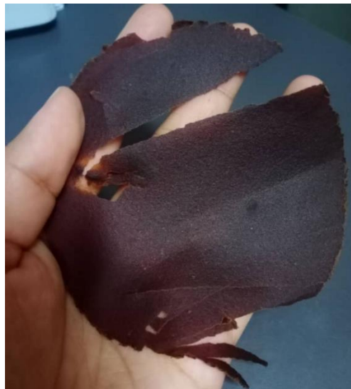
Figure 3. Ruptured banana peel and corn starch film incorporated with cinnamon EO
