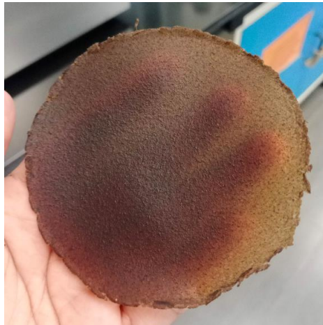
Figure 5. Texture surface of banana peel and corn starch film incorporated with cinnamon EO
