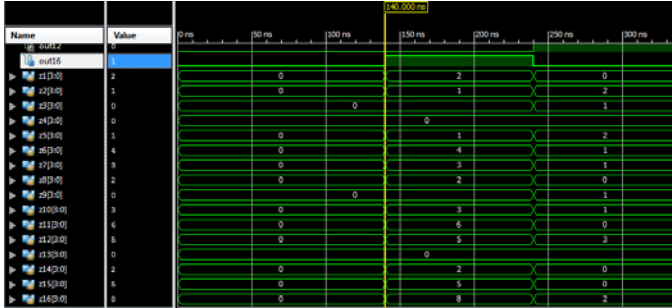
Figure 9 : Timing diagram of comparator 1 form Isim simulator
