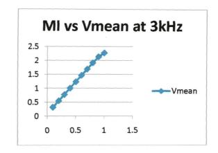
a) Vmean of the first quadrant with R load at 3kHz
