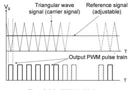
Figure 3: Pulse Width Modulation
