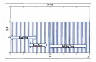
Figure 12: PWM signal output from FLC for Vref= 5 Volt.
