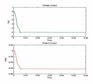
Figure 11: Output Voltage and Current from Buck-Boost Converter using FLC Vref= 5 Volt.
