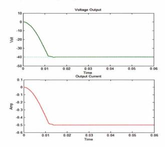
Figure 13: The Output voltage and Current Vref= 40 Volt using FLC Buck- Boost converter.
