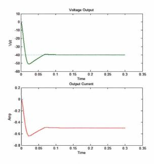
Figure 17: Output Voltage and Current from Buck-Boost Converter using PIC Vref= 40 Volt.
