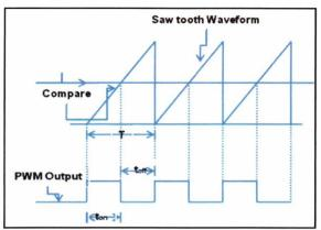
Figure 6: The change of duty cycle of PWM generator.
