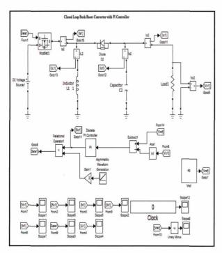
Figure 10: A Simulink model of PI for Buck-Boost Converter.
