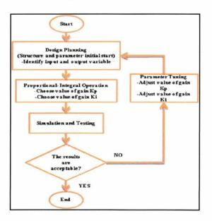
Figure 8: Illustrate Matlab Proportional Integral steps flow.
