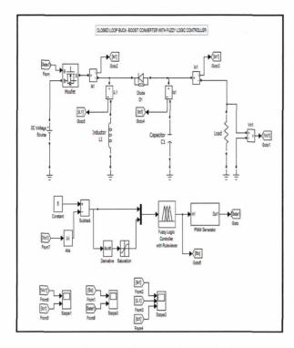
Figure 9: A Simulink model of Fuzzy Logic controller for Buck-Boost Converter.
