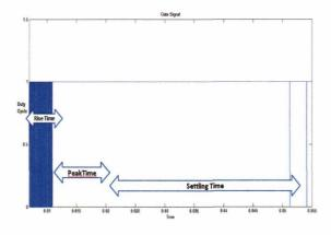
Figure 16: PWM signal output from PIC Buck-Boost converter for Vref= 5 Volt.
