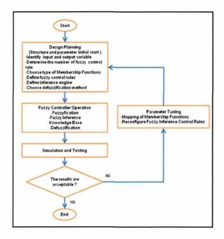
Figure 3: Illustrate Matlab Fuzzy Logic Toolbox steps flow.
