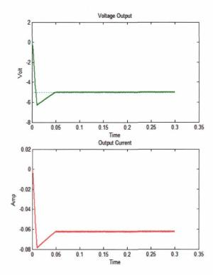
Figure 15: Output Voltage and Current from PIC Buck-Boost Converter using PIC Vref= 5 Volt.
