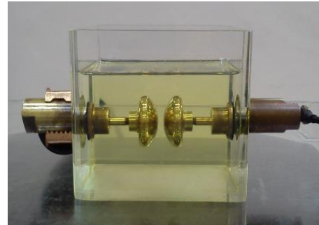
Fig 3. Test cell filled with test sample
