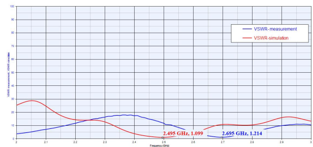
Figure 11 .VSWR of Hexagonal Patch Slit-back Antenna
