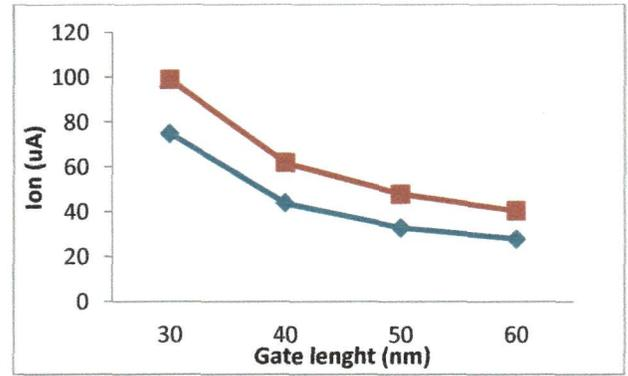
Fig. 7:  $I_{ON}$  for a MOSFET (■) and a FinFET (◆) for variation in length of gate.
