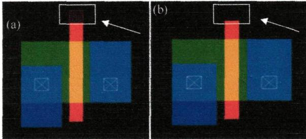
Fig. 2: Layout of generator MOSFET (a) and FinFET (b) that different at the gate
