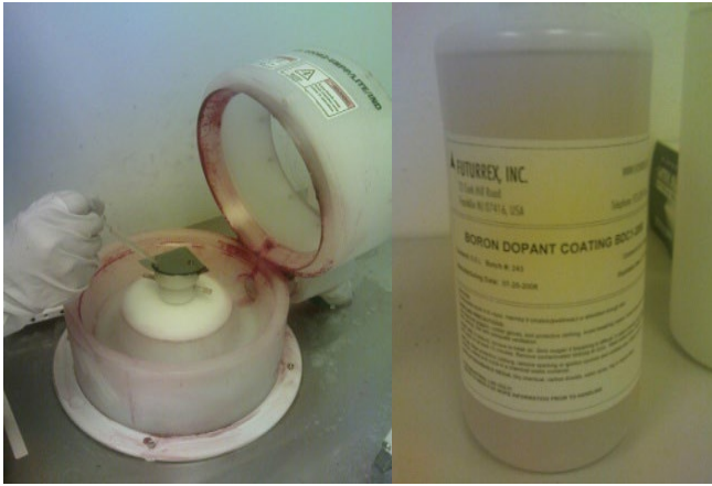
Fig. 3. Spin Coater and P-type Liquid Dopant
