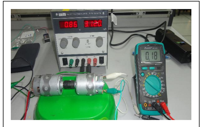
Fig. 6: Testing speed and voltage generation
