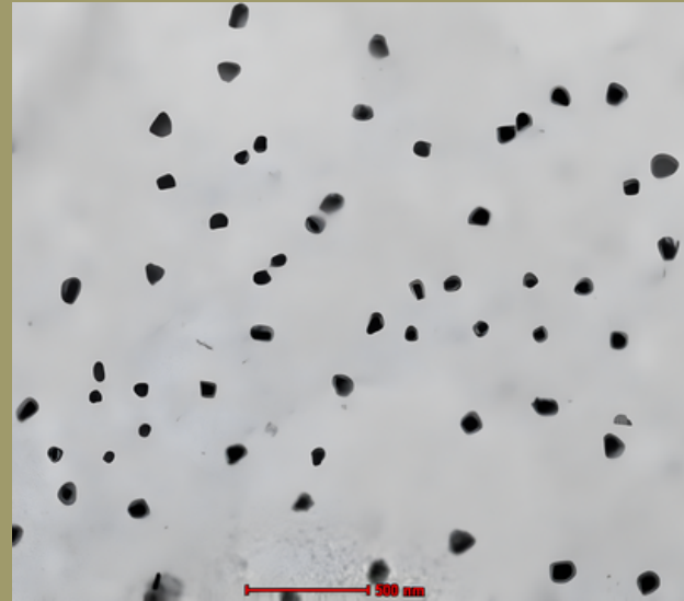
Transmission electron microscopy (TEM) micrograph of the obtained nanoparticles with cuboidal shapes.
