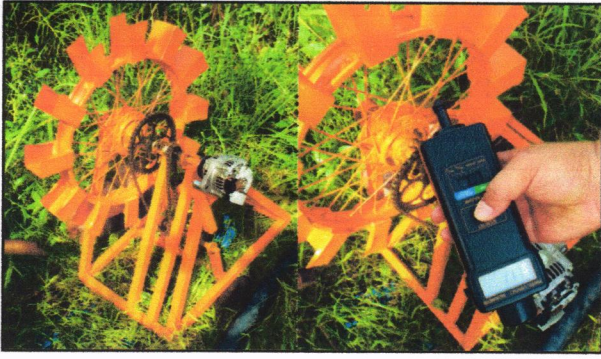
Figure 2. A prototype water wheel turbine
