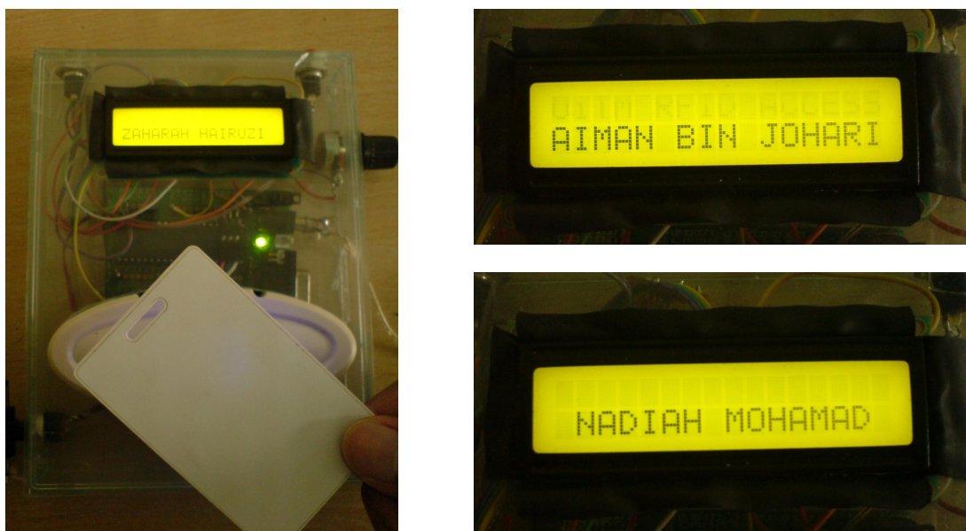
Figure 4.3: LCD displaying students' name when the RFID is tapped
