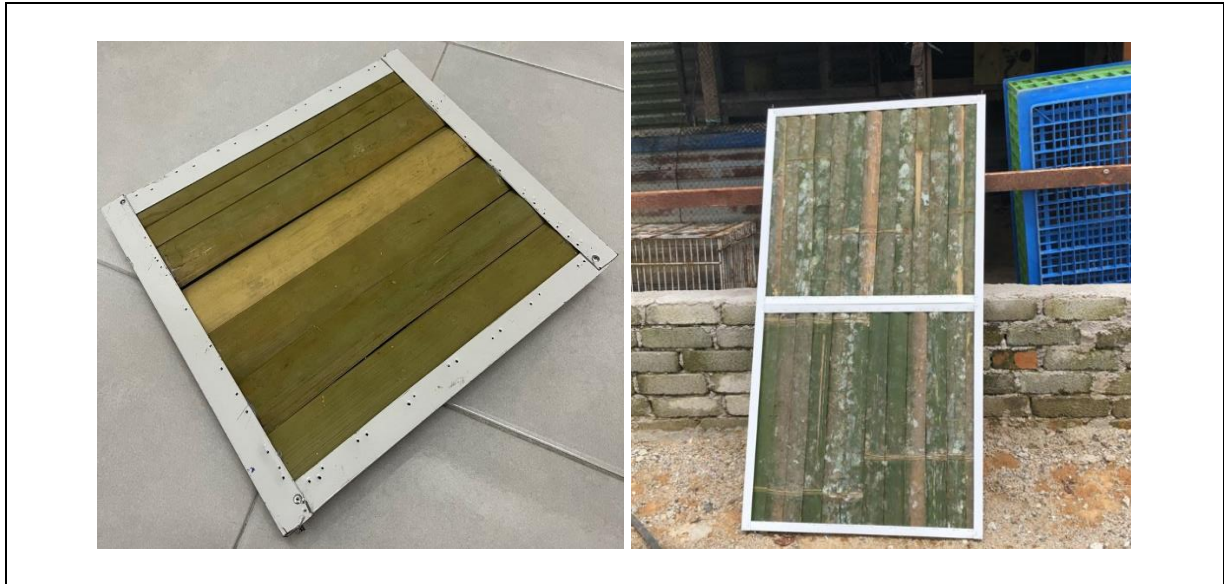
Application Of Bamboo As A Ceiling Panels
