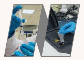
Left: A laboratory staff demonstrating accurate way of filling the Zetasizer cuvette with sample. The cuvette can be bought from the laboratory at a reasonable price. Right: Loading of the cuvette into the Zetasizer. The solution's particle size and zeta potential will be measured on operator's click.
