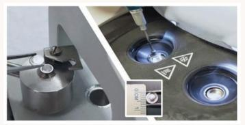
Left: Sample is placed inside the pan and covered with a lid before it is sealed through mechanical clamping. Middle box: A sealed DSC pan. The single use pan and lid can be bought from the laboratory at a very reasonable price. Right: Sealed pan with sample to be tested is placed on
