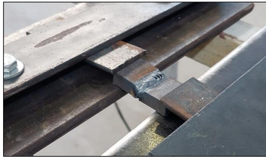
Figure 4: Welding samples for a hardness test and microstructure inspection
