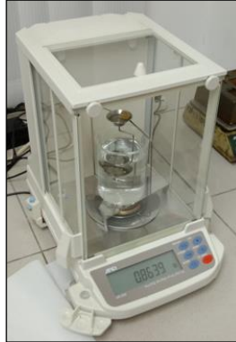
Figure 5: Density measurement using Archimedes' principle
