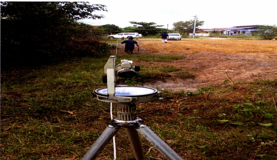
Figure 2 : This diagram shows the compass that had being used during process of measuring the position of land bearing
