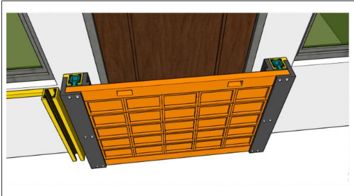
Flood Barrier Safety Door
