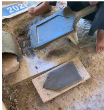
Figure 5: The Wet Green Tiles Placed on the Pallet (Field Observation, 2021)
