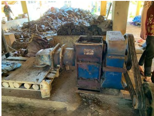
Figure 4: Machine used to smooth the clay (Field Observation, 2021)
