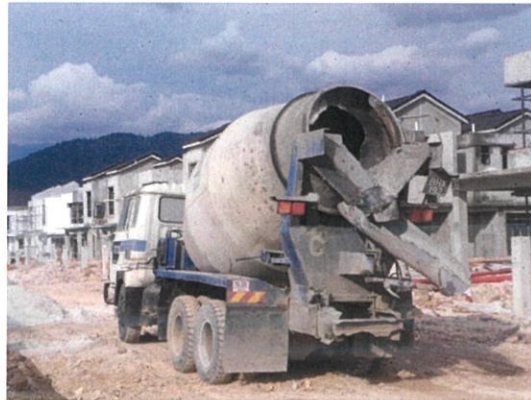
Figure 3.54: Concrete Mixer Truck.
