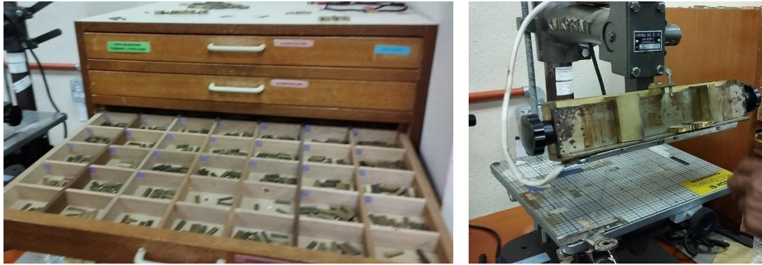
Figure 62: Find the alphabets (glod blocking) for the book title and the blocking press
