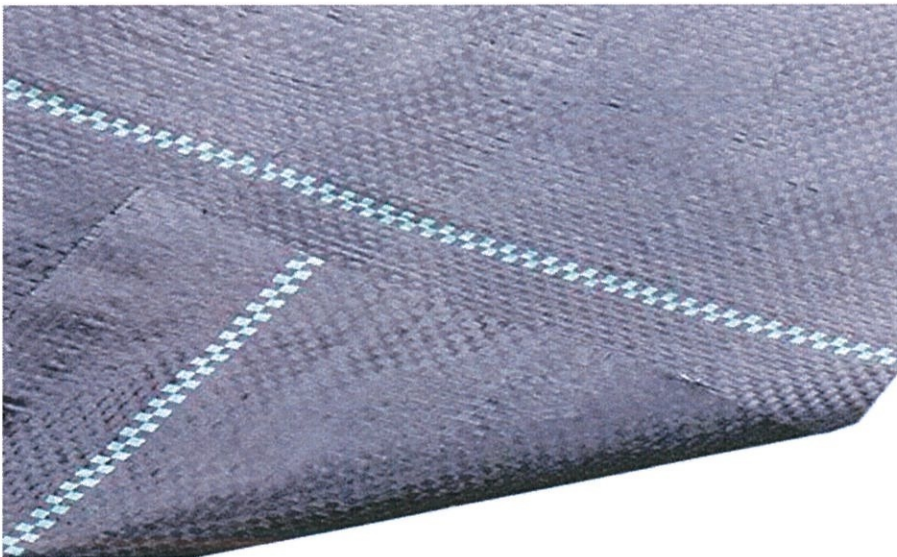
Figure 3.8 Geotextile fabric membrane
