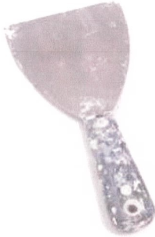
Figure 3.2.8: Putty trowel scraper
