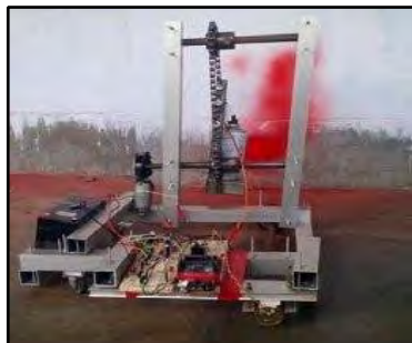
Figure 3: Automatic wall painting robot (Source: Keerthanaa et al., 2013)
