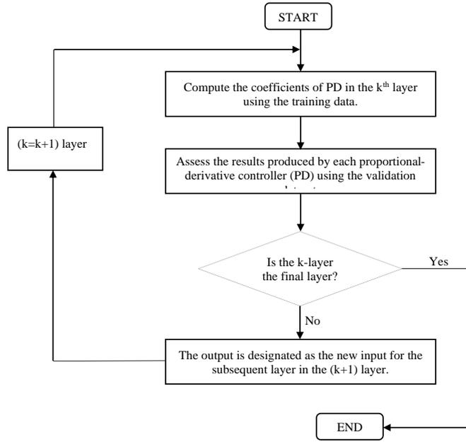
Figure 1. Group Method of Data Handling model framework
