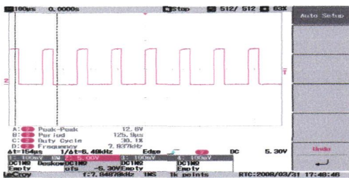
Figure 34: Driver IR2110 waveform
