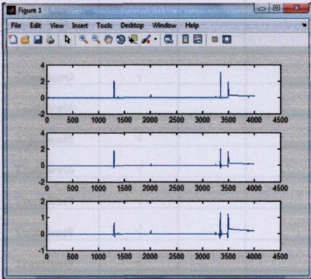
Figure 10: Multilevel Decomposition Using Daubechies3
