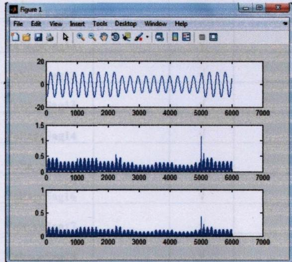
Figure 12: Example of Voltage Sag Analysis
