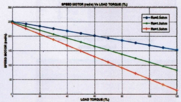
Figure 8: Torque-speed characteristics for three different armature resistance for Separately Excited DC motor
