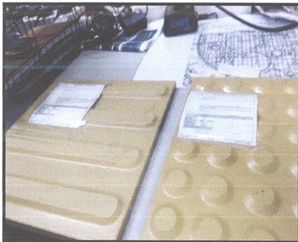
Figure 3.1.2(e) : Sample of rubber tactile tiles receives by QA/QC engineer
