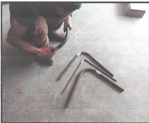
Figure 3.3.2(k) : Checking any cracks
