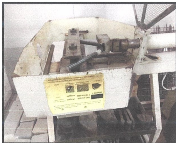
Figure 3.3.2(l) : Re-bending the rebar after heating process
