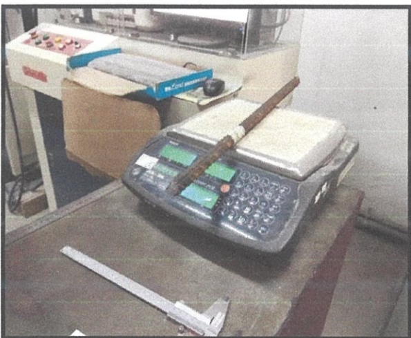
Figure 3.3.2(g) : Weighing the rebars
