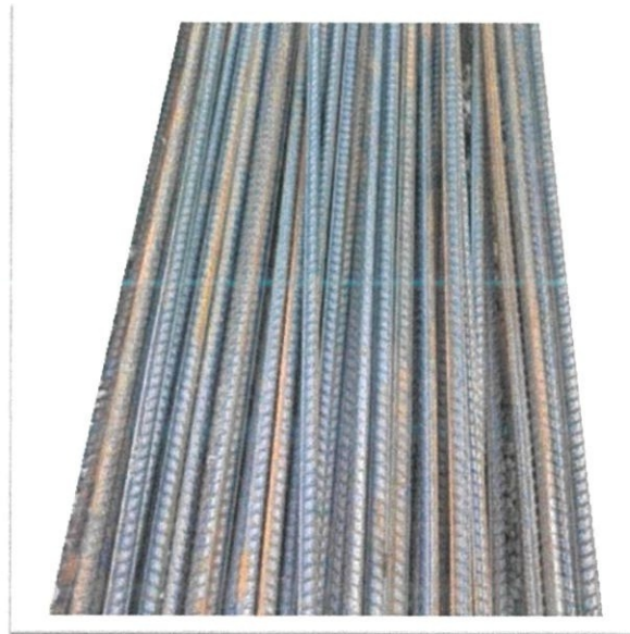
Figure 3.29 : Y12 reinforcement steel
