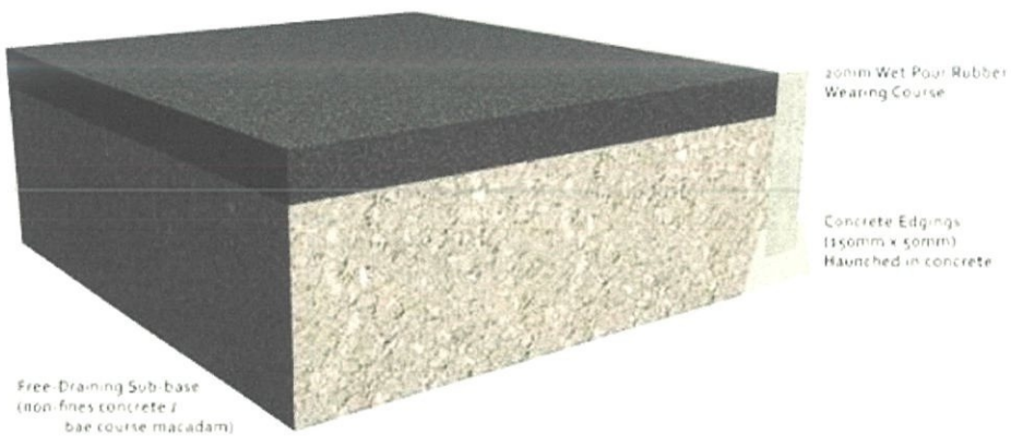
Figure 3.17: The wearing course and binder course layer
