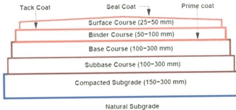
Figure 3.16: The pavement layer
