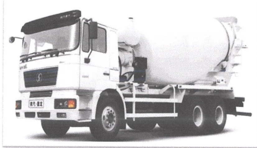
Photos 3.3 : Concrete Mixer Lorry
