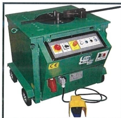
Photo 3.15 : Shows the steel bar bending machine
