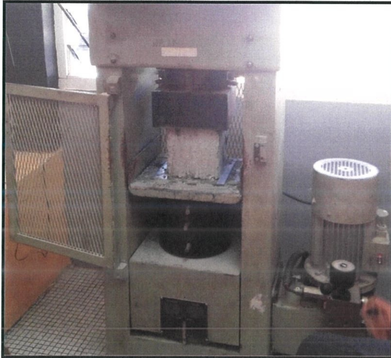
Photo 3.6 : Shows the concrete cube Grade 35 being tested
