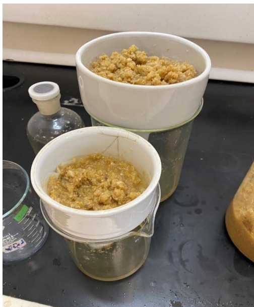
Figure 3.4 Washing and filtration
