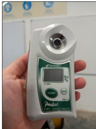
Figure 3.2 Atago digital hand-held “pocket” refractometer (PAL-3)
