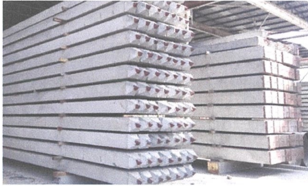
Figure 3.3 : Initial and extension of concrete pile
