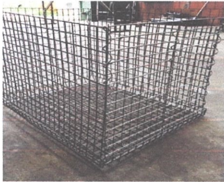
Figure 1: Shows the gabion baskets
