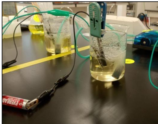
Figure 3.6 EF setup powered by 1.5 V battery.
