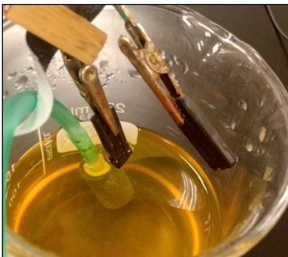
Figure 4.5 Contamination due to rust.
