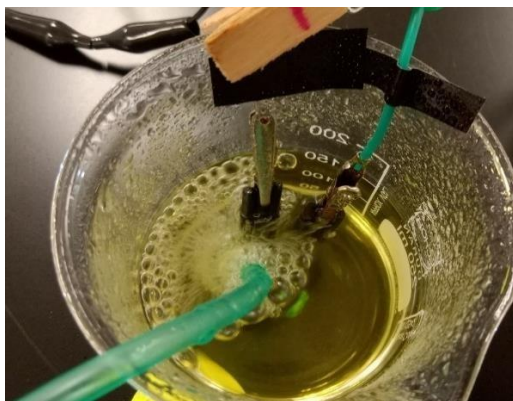
Figure 3.7 Electrodes submerged into beaker.
