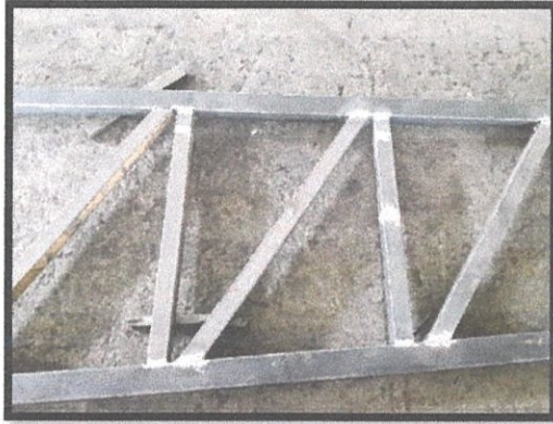
Figure 3. 9: Results of smooth surface after grinding.
