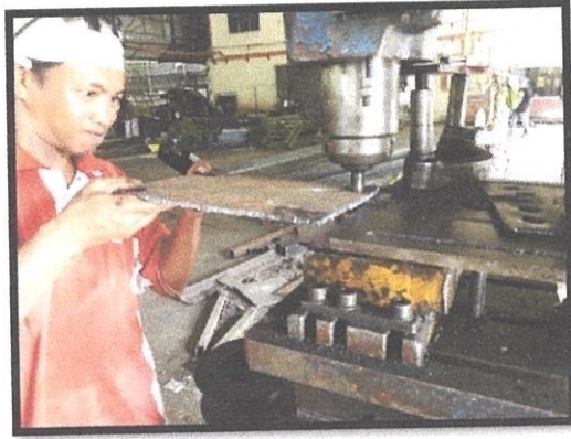
Figure 3. 11: Labor was punching a hole on the plate.
