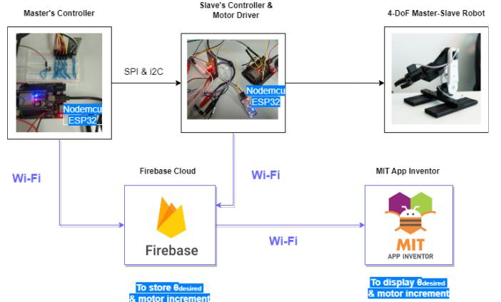
**Fig. 4.** Master-Slave robot monitoring system architecture.
