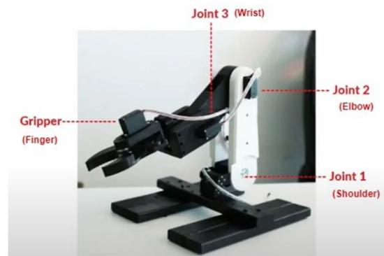
b) The modified design of 4-DOF slave robot.
