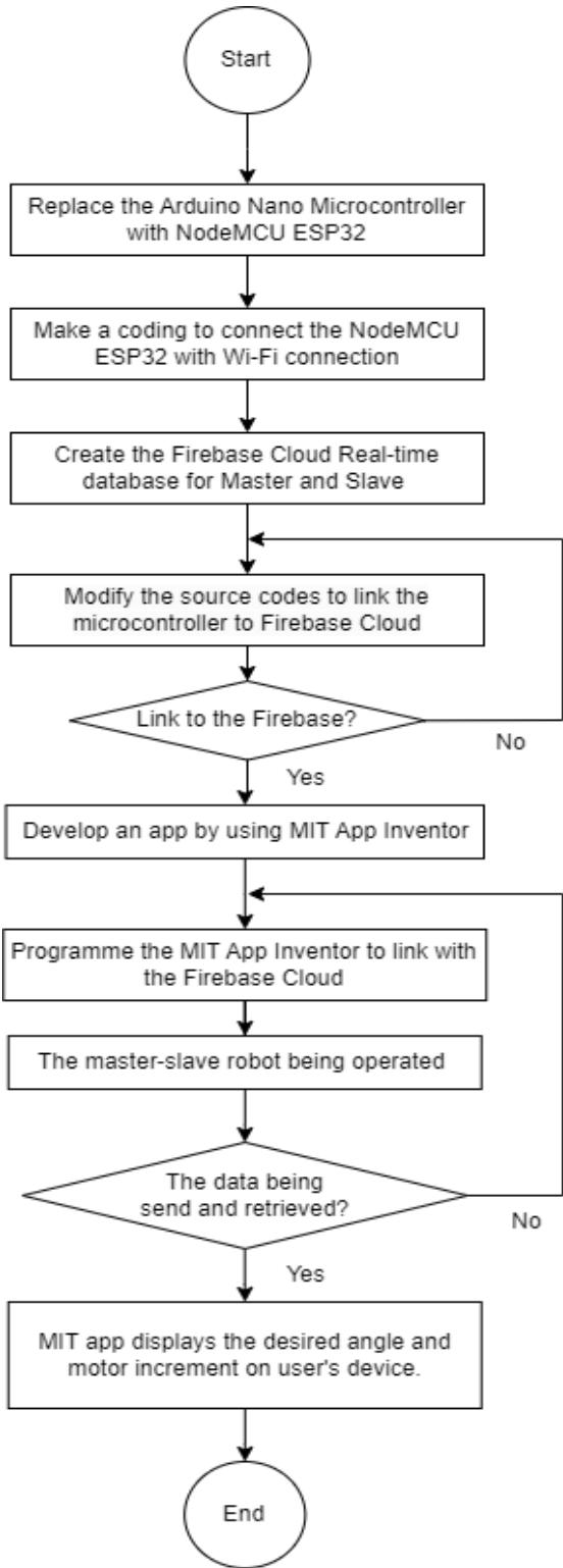
**Fig. 3.** Phase II steps consisting of the programming of different boards, database and MIT App Inventor.
