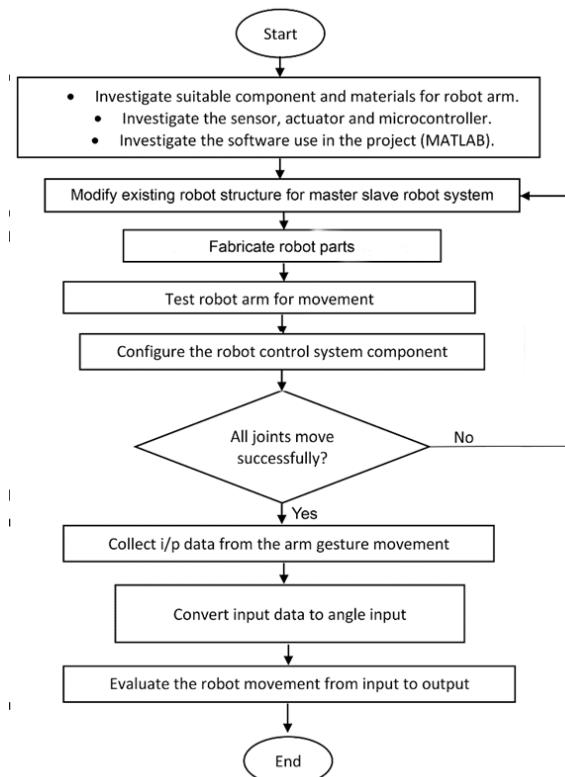
**Fig. 2.** Phase I involving the development of the master-slave robot [14].
