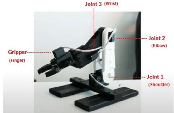
b) The modified design of 4-DOF slave robot.
