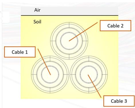
Fig. 3. The completed cable construction using the geometry function in COMSOL Multiphysics.
