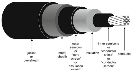
**Fig. 1.** Power Cable Structure [12].
