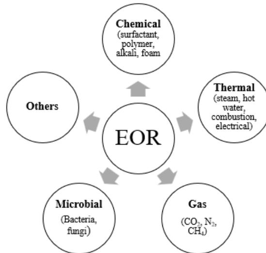
Fig. 1. Different types of EOR operations involving chemical agents
