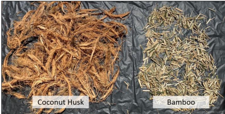
Figure 2: Image of the coconut husk and bamboo residue after being cut and before being ground into fine particles
